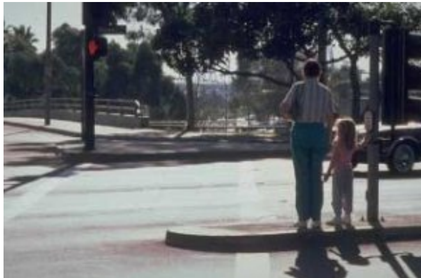
Figure 2-11. Pedestrians crossing road with raised median (FHWA 2005).
